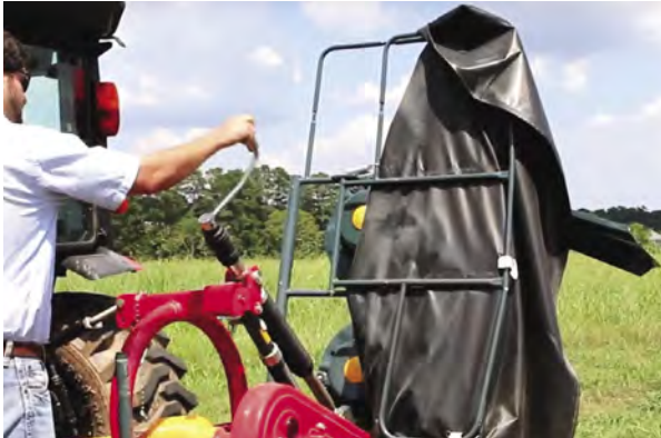
Drum Disc Mower – raise and lower by rotating the handle to change from transport position to working position.
