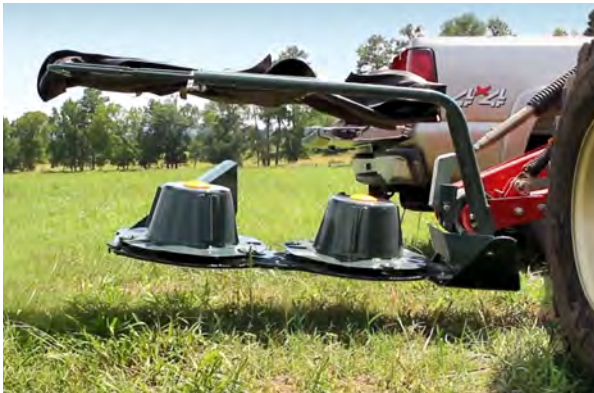
Raise and lower mower arm with the 3-point hitch.
