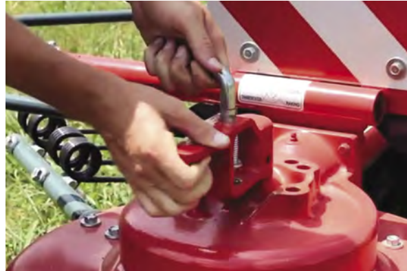
Tedder/Rake Change functions by shifting one lever.
