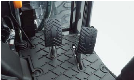
Side-by-side forward/reverse pedal
